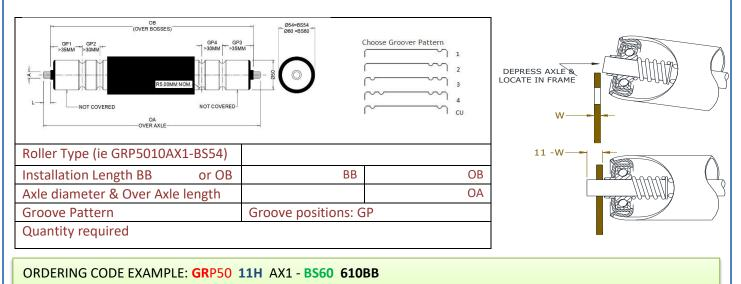
Roller Type ¦ Axle Size ¦ Sleeve Diameter ¦ BB (Installation Length) or OB if you specify Over Bosses
