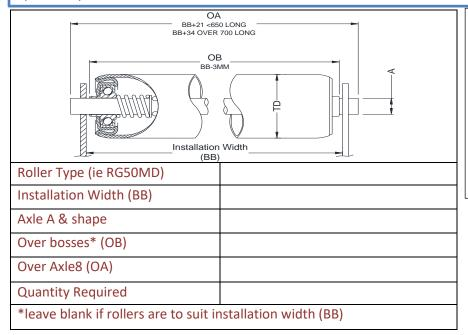
Bearing housing: steel swaged
